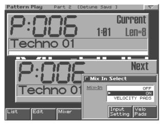
2. Continuing to hold down [MIX IN], press [F6 (Velo Pads)] or turn [VALUE] to select "VELOCITY PADS."
